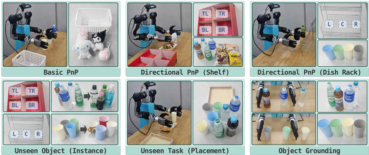
Figure 13: OpenArm humanoid benchmark. We visualize the initial setup for six tasks for evaluating versatility in humanoid manipulation: Basic PnP , Directional PnP (Shelf) , Directional PnP (Dish Rack) , Unseen Object (Instance) , Unseen Task (Placement) , and Object Grounding .
