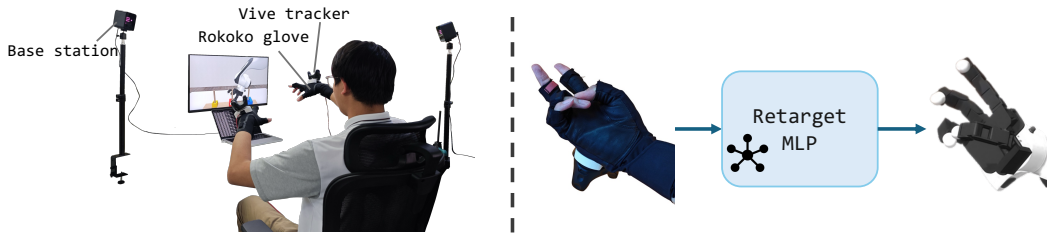
Figure 3: Human demonstration data collection system. The left figure shows the overall teleoperation system. A Rokoko glove is used to capture hand poses, while an HTC Vive tracker is employed to track the wrist pose. The right figure shows that a retargeting mapping is trained to convert human fingertip poses into joint configurations of the Allegro hand.
