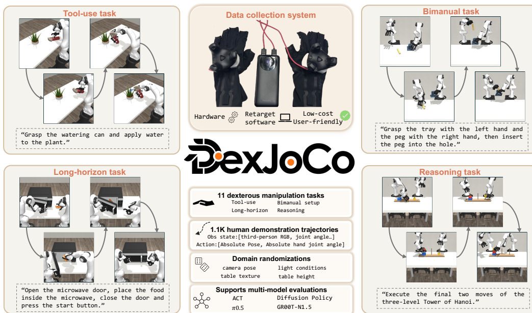
Figure 1: Overview of DexJoCo. DexJoCo is a dexterous manipulation benchmark with a toolkit for data collection and policy evaluation, covering tool-use, bimanual coordination, long-horizon execution, and reasoning. It includes 11 tasks, 1.1K human demonstration trajectories, and supports trajectory replay under domain randomization for robustness evaluation.
