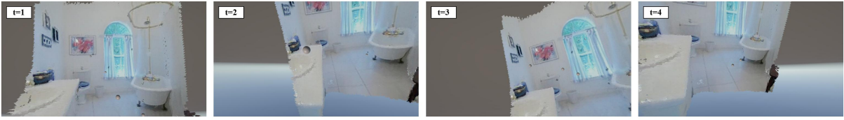
Figure D Unity object interaction. We load the reconstructed mesh into Unity and interact with the scene using standard engine collision and physics components. The four frames show temporal progression from t = 1 to t = 4 ; stable contact with reconstructed surfaces indicates that the exported triangle mesh is directly usable for interactive applications, rather than only for image rendering.
