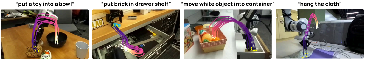
Figure 8 MolmoMotion trajectory prediction on real-world scenarios. Predicted future 3D object trajectories on a held-out scenario after finetuning MolmoMotion on DROID videos. MolmoMotion can plan accurate object trajectories for various robotic manipulation tasks.
