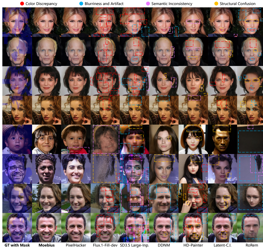
Fig. 9: More qualitative comparison on portrait scenes (CelebA-HQ and FFHQ). Rows 1–4: CelebA-HQ; rows 5–8: FFHQ. Moebius excels in facial restoration, maintaining superior structural integrity and skin texture fidelity compared to other methods. Specifically, Moebius provides sharper and more coherent results, avoiding color discrepancies on face (row 1), reducing blurriness and artifacts at mouth and ear (rows 2 and 3), suppressing semantic inconsistencies in hair (rows 4 and 5), and preventing structural confusion at teeth and background (rows 6, 7 and 8).
