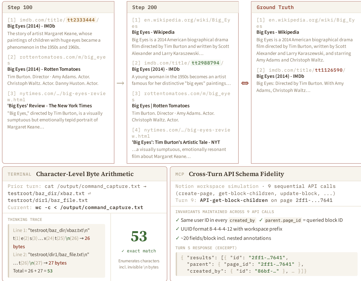
Figure 13: Micro-level fidelity improvements during RL training. Top: Search domain: evolution of a single sample across RL steps. URL identifiers, source diversity, and snippet specificity all improve, despite occupying a tiny fraction of total output tokens. Bottom left: Terminal domain: the model performs exact byte-level arithmetic by enumerating characters including invisible newlines. Bottom right: MCP domain: the model maintains cross-turn schema consistency (user IDs, parent-child references, UUID formats) across nine Notion API calls.
