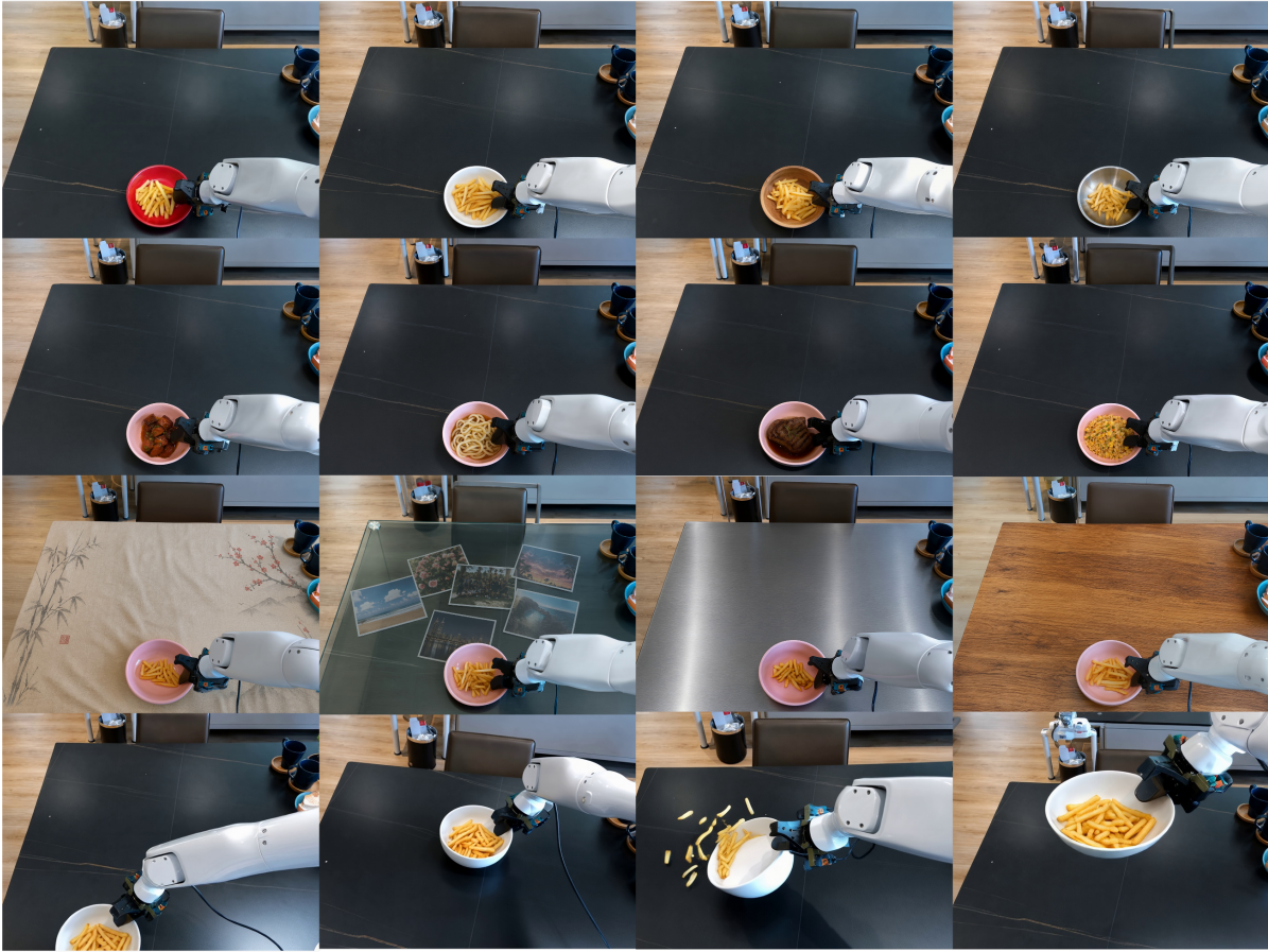
Figure 15: OOD generalization cases. From top to bottom, the rows evaluate generalization to object color and container appearance, object content changes, background and table-surface changes, and action-outcome variation covering both successful and failed executions.
