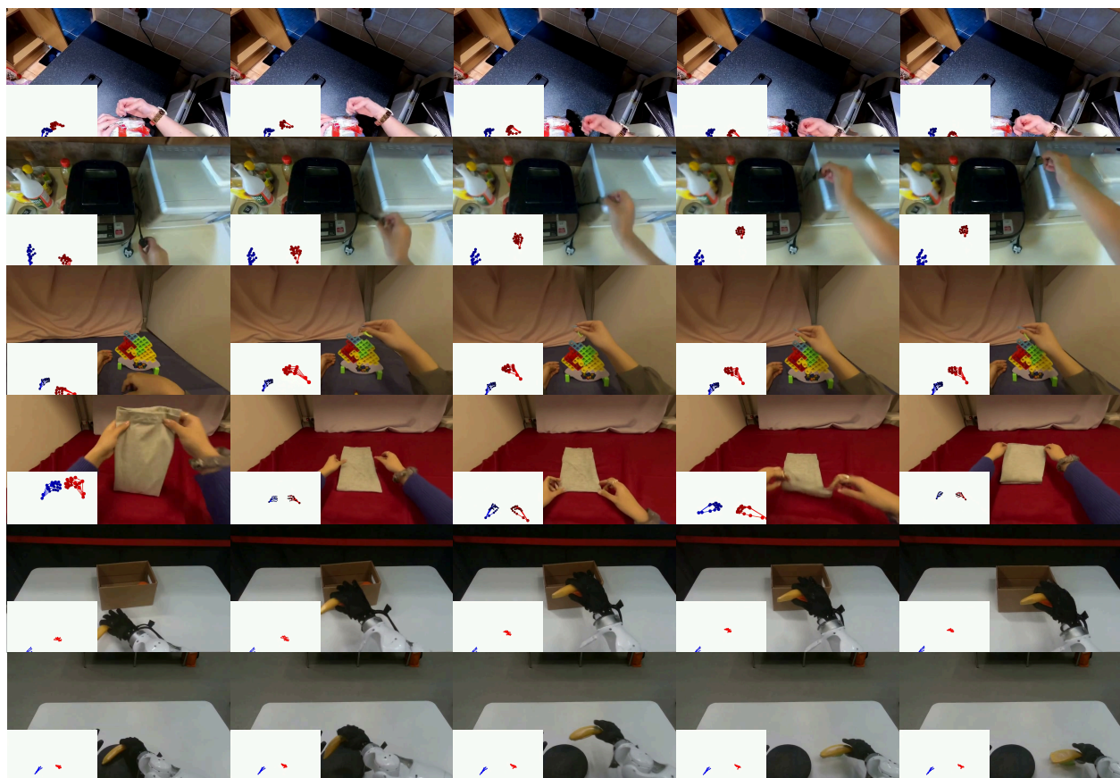
Figure 6 Qualitative Results of RynnWorld-Teleop. Our model effectively maps a single hand-gesture stream to both human and robotic embodiments. By pre-training on large-scale egocentric human videos, RynnWorld-Teleop absorbs rich manipulation priors and successfully transfers this knowledge to robotic execution. The synthesized videos maintain high fidelity and temporal coherence.
