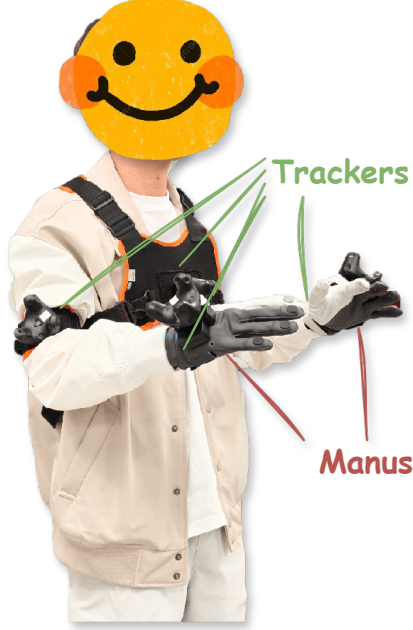
Figure 11 Operator setup for real-world data collection.
