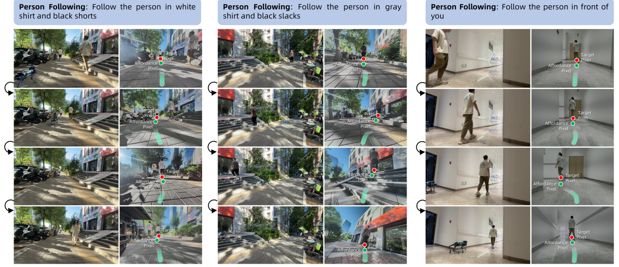
Figure 14 Person-Following Deployment. Outdoor tracking under pedestrian distraction, stair-climbing following, and indoor corner-rounding with temporary occlusion.
