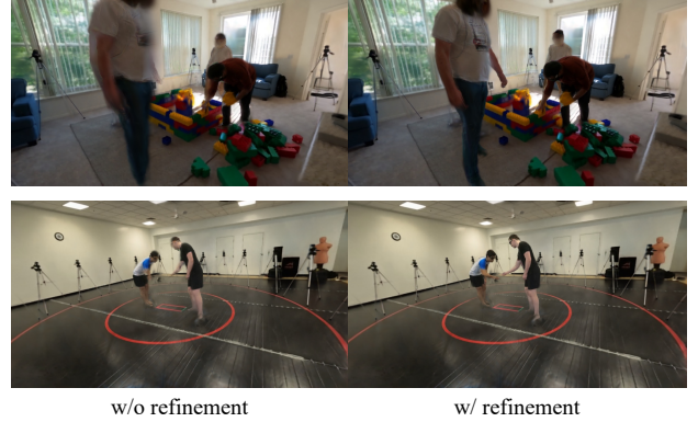
Fig. S5. Effect of multi-view pose refinement. Without refinement (left), inaccurate SMPL poses cause blurry or semi-transparent body parts. With refinement (right), poses are corrected via cross-view triangulation, producing a sharper human reconstruction.
