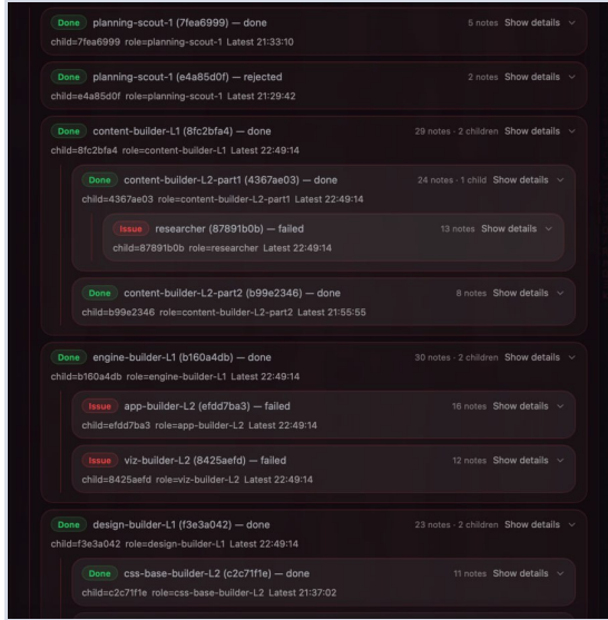
Figure 3: Task-tree view of a live Ouroboros session: nested planning and acting roles with per-node status, note counts, and child counts.
