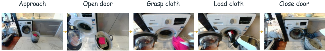
Figure 16 Temporal anchors for contextual teaching: opening the door enables loading, and closing it completes the procedure. These transitions align a teaching example with progress in a later execution.
