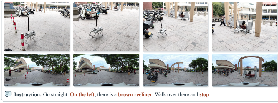
Figure 5: Real-world navigation. PanoVLN deployed on a quadruped robot and transfers to real-world instruction following without scene-specific fine-tuning.
