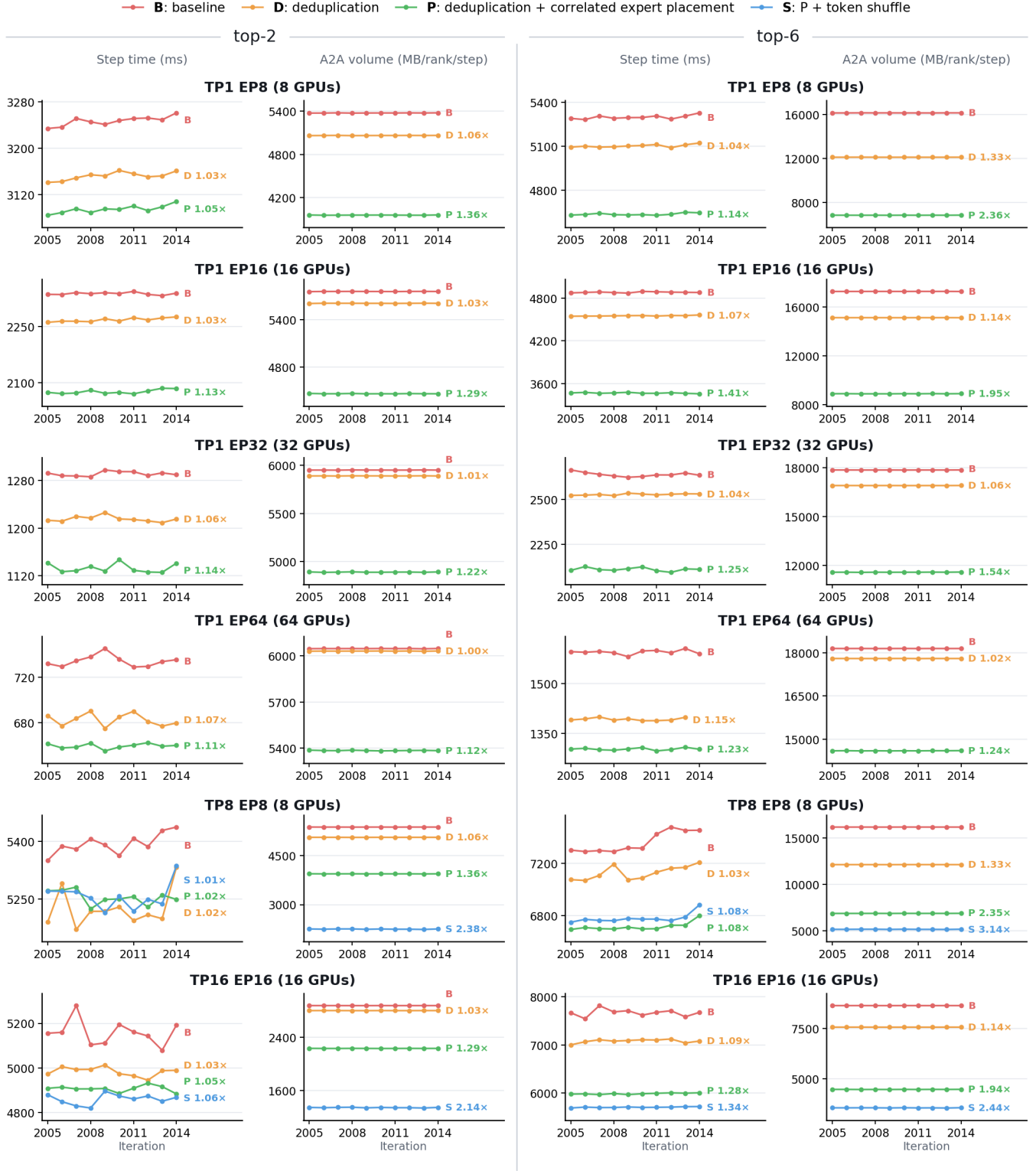
Fig. 12: Step time (left) and A2A volume per rank (right) for the ten measured steps of each configuration, after the four warm-up steps. Data point labels give the ratio of the baseline median to the median of that configuration.
