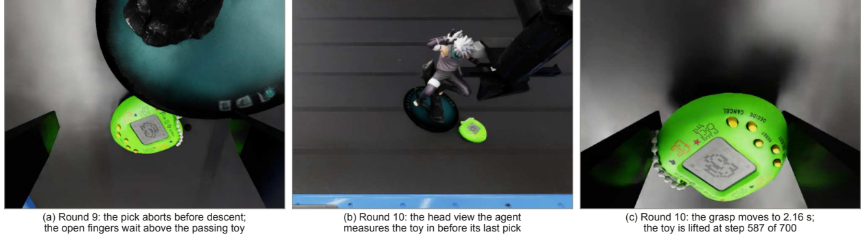
Figure 7. Match and pick from conveyor, layout 4: time, not position. (a, c) right wrist camera; (b) head camera, cropped. (c) is the last frame of the video, since the episode ended during the lift.
