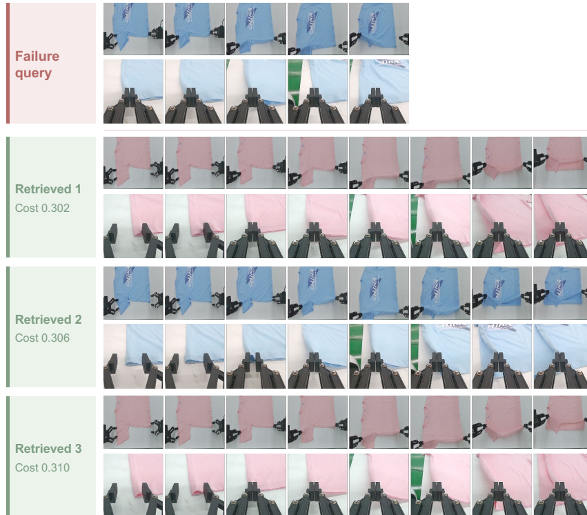
Figure 17 Visualize the retrieval effect in Clothes Folding. The top row shows a failure segment in which the robot attempts to fold a T-shirt in half but fails to grasp its right corner with the right gripper. The following rows below show the corresponding retrieved segments. With an appropriate feature representation, FERT retrieves the same critical step across clothes of different colors.
