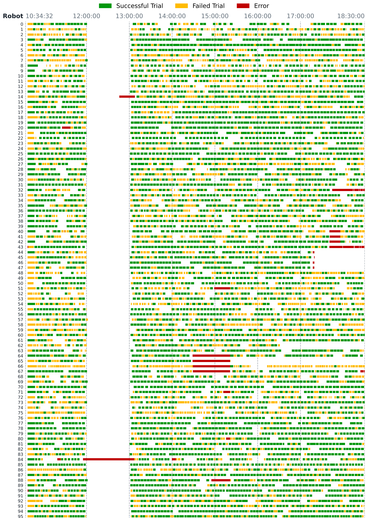
Figure 13 Detailed per-robot trial timelines during a 96-robot training run. Successful trials, failed trials and system errors are marked separately; blank intervals include environment resets and operator breaks.
